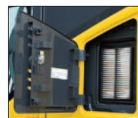
External air conditioner filter
