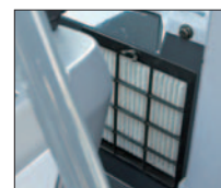
Internal air conditioner filter
