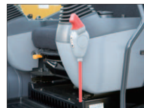
Lever shown in lock position
